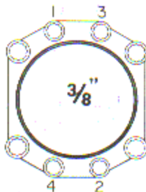
Figure 3. Proper Sequence of Tightening Cylinder Base Nuts
