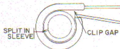
Figure 2. If split sleeve is used, locate split approximately 180° from gap in clamp, as shown.
