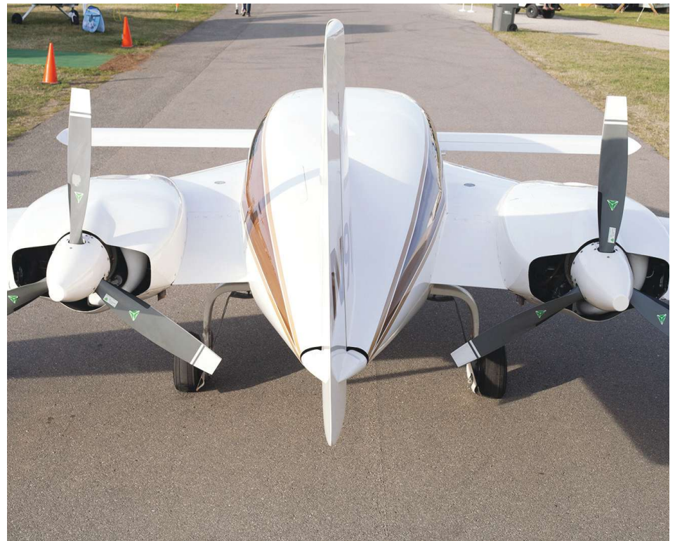
The engines are mounted closer than normal to centerline, which reduces asymmetric thrust with a dead engine.
