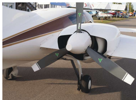
The 160-hp, fuel-injected Lycomings are burning 6 gallons each at 175 ktas, or 8 gallons at 185 ktas.
