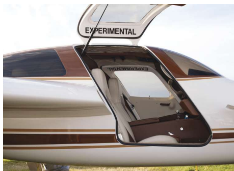
The XL cockpit/door dimensions, which are larger than many “normal” twins, were retained on the V-Twin.
