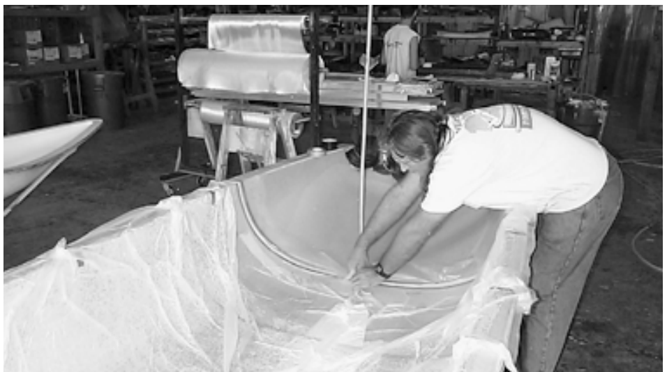
Lambert Kneifel attaches vacuum bag umbilical line to XL fuselage mold part.
