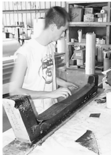
Charlie McElyea fabricates XL-5 drop-down keel cover using carbon fibre BID.
