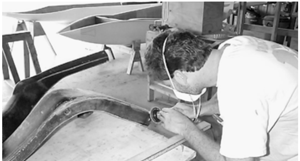
Chad Holland applies carbon bid torsional wrap to XL-5 retract gear leg.
