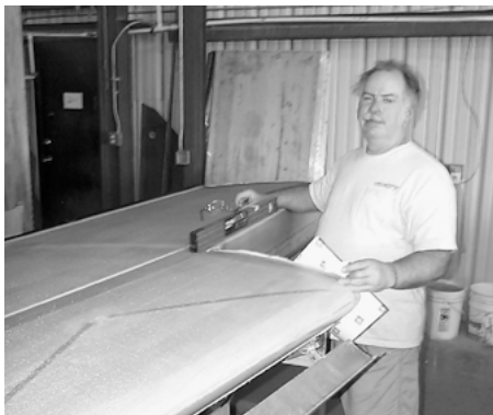
Jim Parrot covers wings with triax cloth as part of the Fastbuild Wings Option process.
