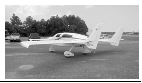
increased to 34 feet and the ailerons have been moved as far outboard as possible.
