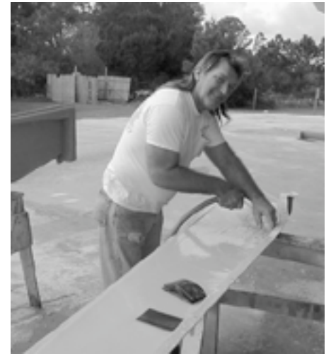
Lambert Kneifel working on new mold of center section keel
