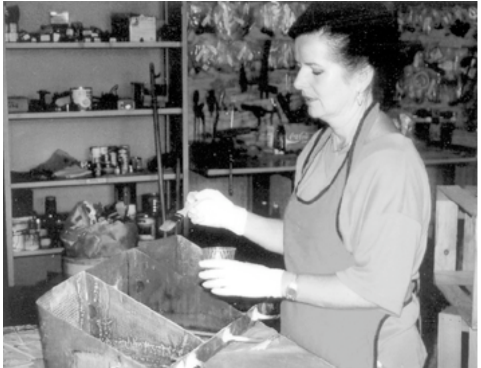
Ursula Wiehl working with epoxy on the Velocity's sump tank
