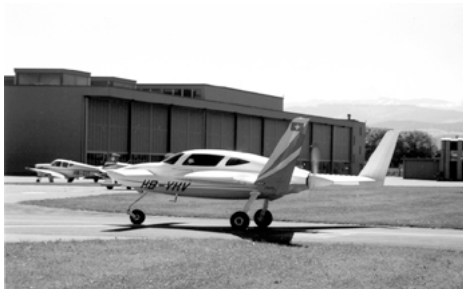
The Velocity 173FG HB-YHV is powered by a Lycoming IO-360 (200 HP) and pushed by a Muehlbauer MT constant speed propeller
