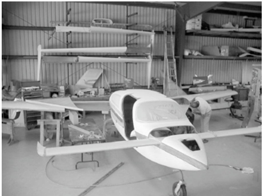
Bob Wood's Velocity XL FG with a set of the new Brazilian wings being installed.
