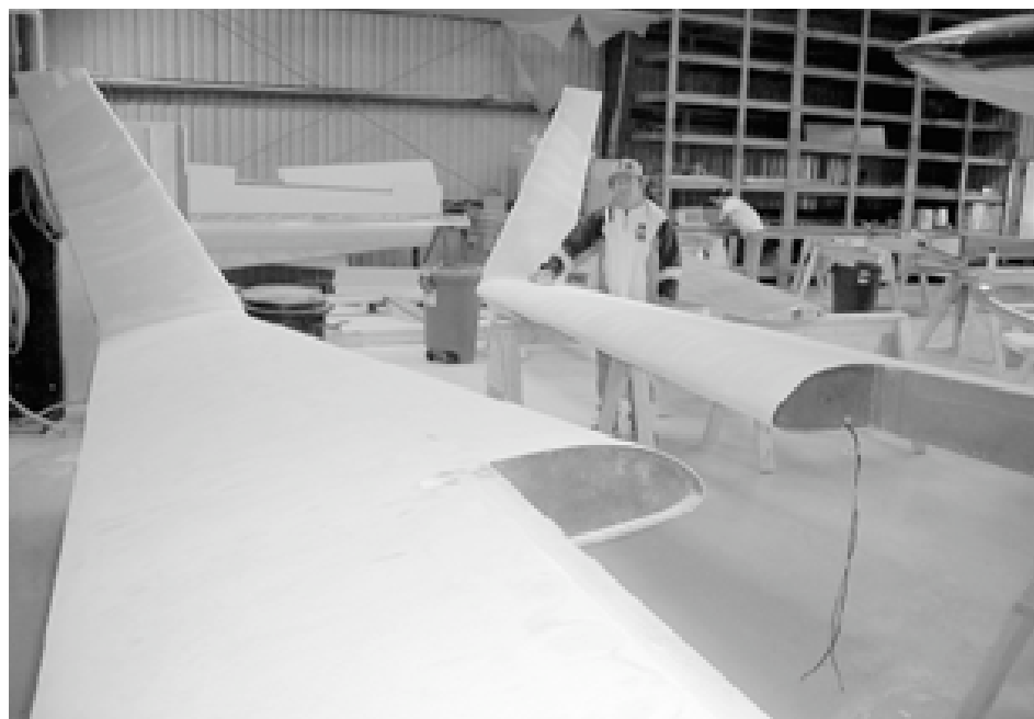
The photos above and below show "Fast Build" wings under construction at the factory
