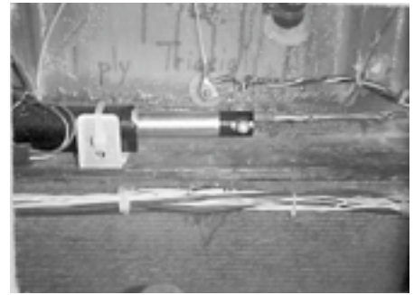
Jack's electric aileron trim actuator motor installed on his center spar. The photo below shows the trim springs attached to the rod ends.
