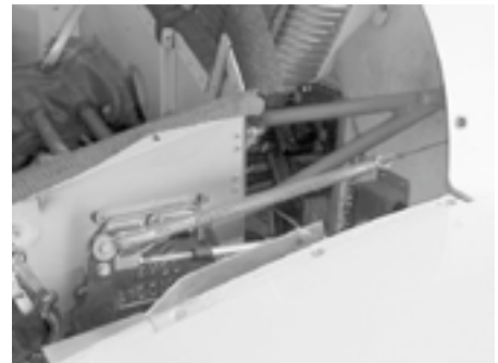
Jack's electric aileron trim actuator motor installed on his center spar. The photo below shows the trim springs attached to the rod ends.
