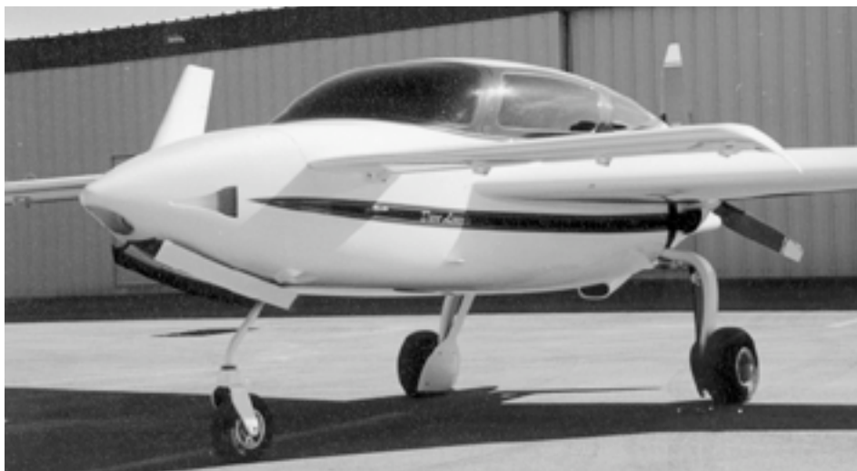
Lincoln's air conditioned Velocity "Dee Dee", has a Franklin 220, MT prop, dual light-speed ignition, dual electrical, Terra avionics, color moving map GPS, and much more.
