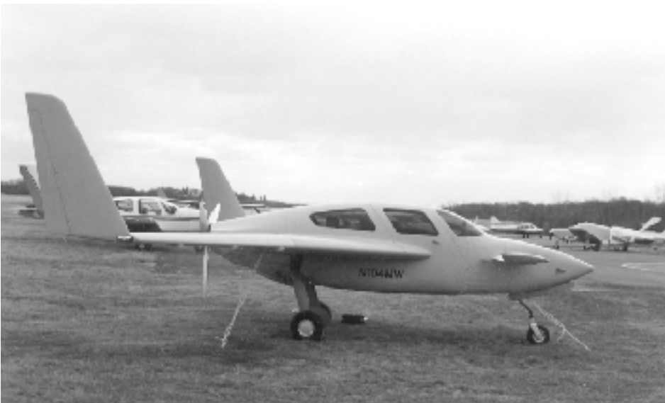
N104MW parked just after her maiden voyage. Mike Watson's Velocity 173 RG is powered by a Franklin engine with an Ivo Prop
