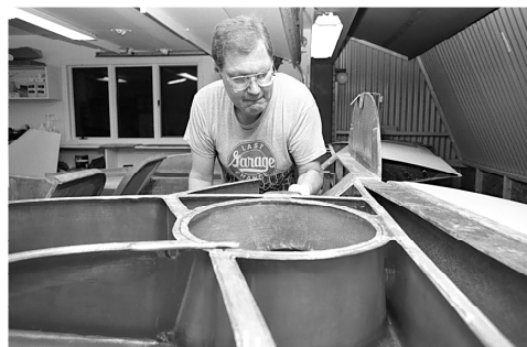
Finish-sanding Completed cap strips
