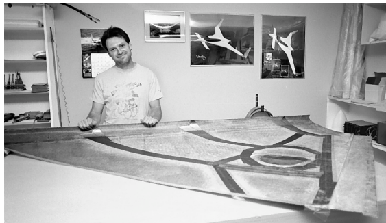
Scott Brown duct-tapes top strake in preparation for lay-up of the 2 BID
