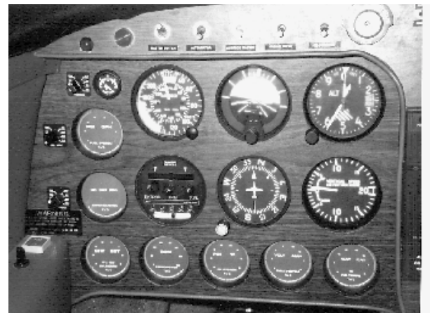
Upper left side panel shows red lights for canopy & speed brake warning lights.
