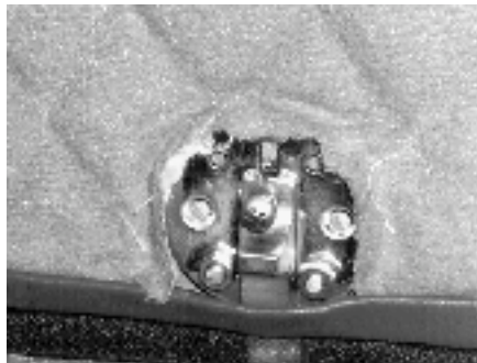
Forward canopy latch with micro switch to turn off red light when latch is engaged
