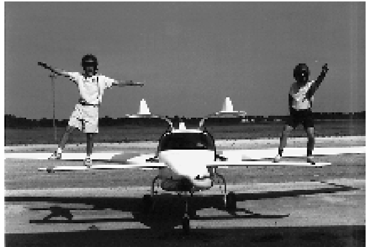
Jeff Baker and Martin Hadley have some fun demonstrating the incredible strength of the Velocity's Canard on the factory prototype 173 RG Elite.
