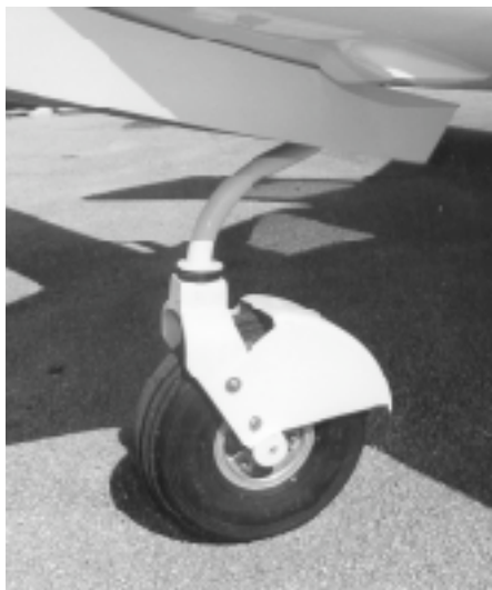
Phil Corso's custom made nose wheel "rock guard"
