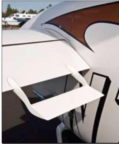
A fixed position trimtab, affectionately called the sparrow strainer, provides pitch feedback and increases pitch stability.
