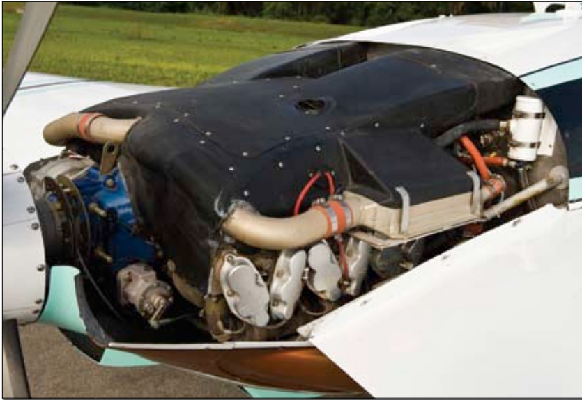
Above: A plenum chamber reduces cooling drag and increases cooling effectiveness. Ensuring that this highly tuned six-cylinder powerplant remains under thermal control is not the work of a moment. Below: A four-blade MT pusher propeller allows for a smaller diameter, resulting in lower tip speeds that increase efficiency, more ground clearance and reduced noise.
