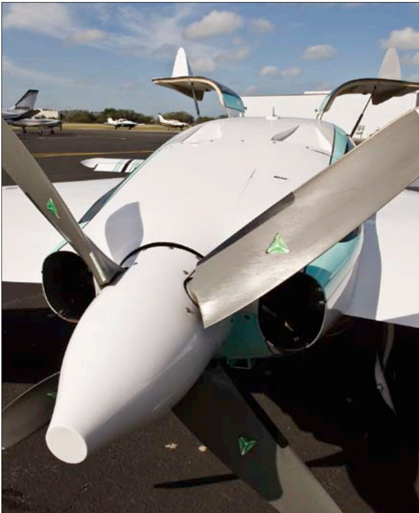
Above: A plenum chamber reduces cooling drag and increases cooling effectiveness. Ensuring that this highly tuned six-cylinder powerplant remains under thermal control is not the work of a moment. Below: A four-blade MT pusher propeller allows for a smaller diameter, resulting in lower tip speeds that increase efficiency, more ground clearance and reduced noise.
