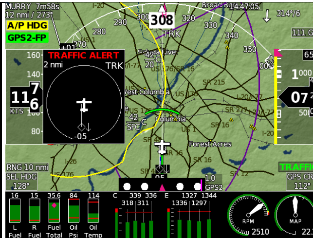
Mode S and ADS-B Traffic with Alerting
