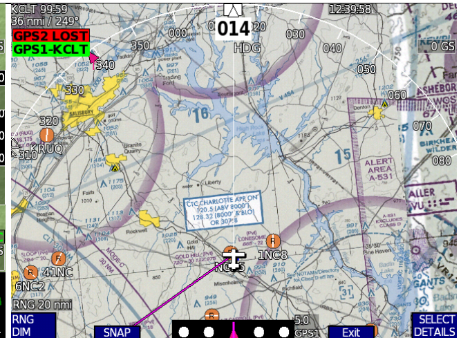
Moving map can display sectional, enroute charts, moving map with airspace, traffic, and weather
