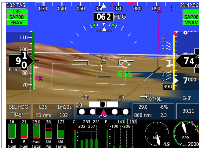
PFD with Synthetic terrain/runways and highway in the sky
