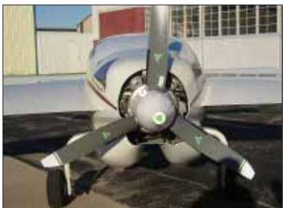
One testbed has been this Velocity, which flies with a three-blade composite MT propeller.
