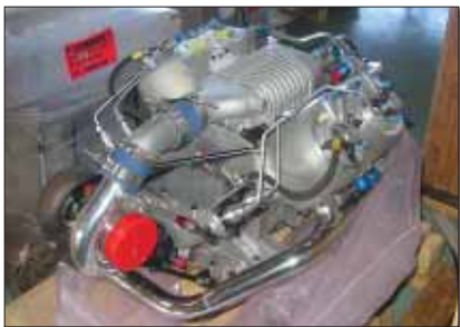
The combined turbo and supercharger layout is neat and tidy. The supercharger helps get the engine started, but the turbo can handle all the flow loads to 100% power.
