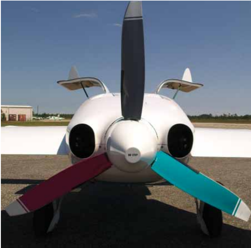
The Dash 5's three-blade MT composite prop is a constant-speed unit optimized for driving the airplane forward instead of dragging it.
