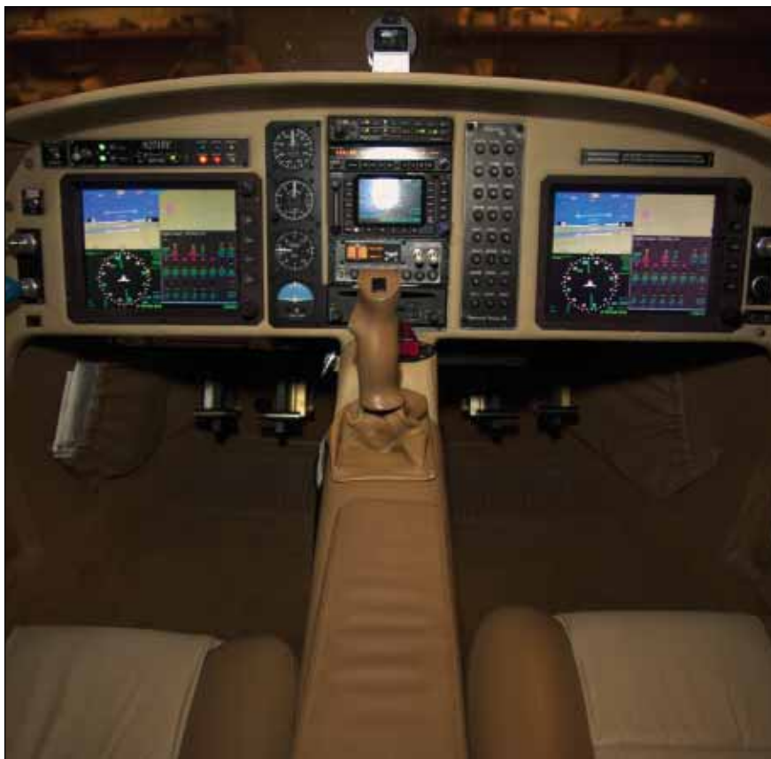
Velocity equipped the Dash 5's panel with a dual-screen installation of Blue Mountain Avionics' EFIS/One system.
