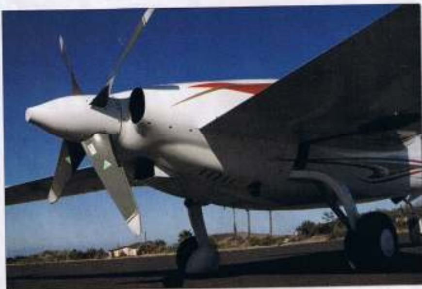
Minimal changes to the cowl were needed to accommodate the TS10-550 engine. A manual cowl flap (center, below the spinner) helps pump more air through the plenum during takeoff and climb.
