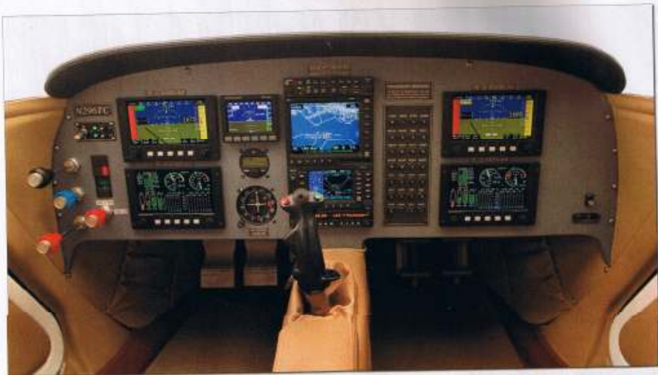
Talk about equipped! N296TC carries a four-screen Grand Rapids suite, backed up by a Dynon D10A, GNS 480, MX20 multifunction display and TruTrak two-axis autopilot. Where's the swimming pool?
