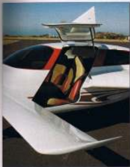
Twin entry doors swing up, a la a Mercedes-Benz SL. Triangular protrusions form the leading edge of the wing strake.
