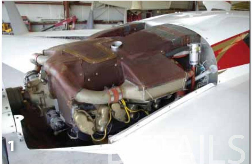
1. A composite plenum chamber grabs cool air from atop the cabin and force-feeds the cylinders and (seen outboard) the intercoolers. 2. Convenient cubbies reside in the leading edge of the strakes behind the door fairing. Don't leave your keys out there. 3. For $8500, any of the current Velocity models can be fitted with retractable gear, which folds neatly into the wing behind the strake. 4. Aside from reangled exhaust-side outlet pipes for the twin Garrett turbochargers, the Continental TS10-550-C engine is as Mobile made it. 5. Twin scoops channel air to the engine compartment.
