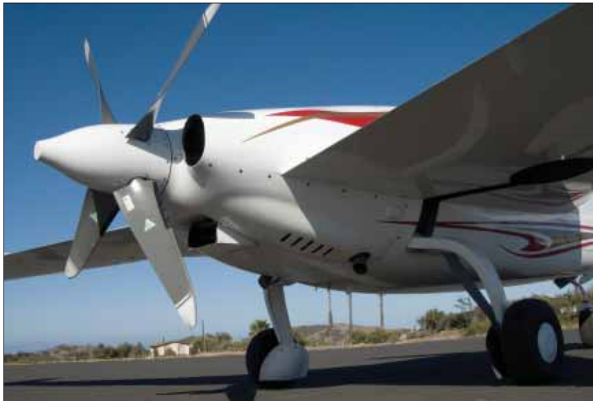
Minimal changes to the cowl were needed to accommodate the TSIO-550 engine. A manual cowl flap (center, below the spinner) helps pump more air through the plenum during takeoff and climb.
