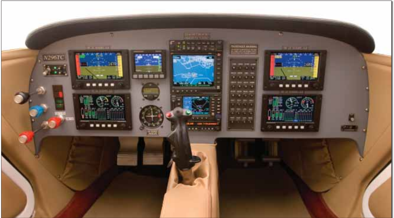
Talk about equipped! N296TC carries a four-screen Grand Rapids suite, backed up by a Dynon D10A, GNS 480, MX20 multifunction display and TruTrak two-axis autopilot. Where's the swimming pool?
